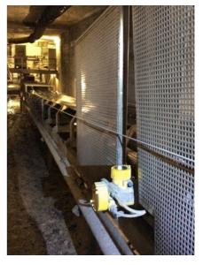
WEIGHTRAC 31 can also be retrofitted to existing conveyor belts. Since it is a non-contact measuring device, wear is not a problem.
