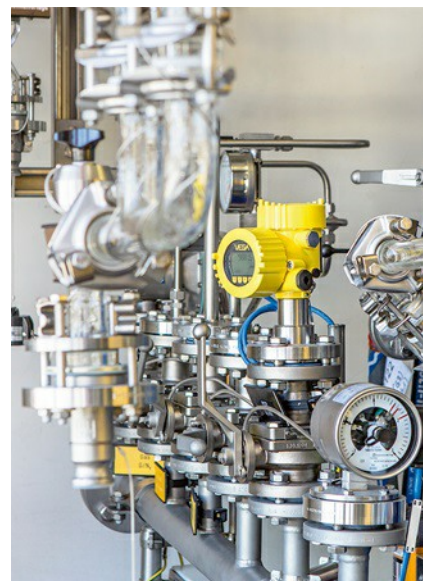
Ensuring simplified qualification: CARBOGEN AMCIS AG uses mostly identical, standardized pressure transmitters.
