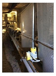
WEIGHTRAC 31 can also be retrofitted to existing conveyor belts. Since it is a noncontact measuring device, wear is not a problem.
