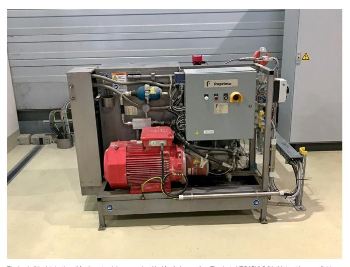
The level of the lubricating oil for the rotary lobe pumps is critical for their operation. Thanks to VEGAPULS 64, this level is now reliably monitored.
