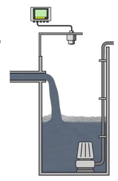
The very good signal focusing of VEGAPULS enables reliable detection of the product surface even in vessels with many internal installations.
