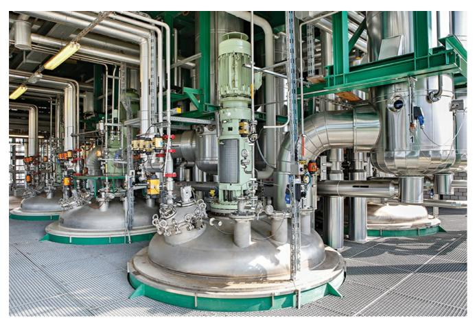
80-GHz radar sensors detect the level reliably even with large stirrers strongly agitating the product surface.
