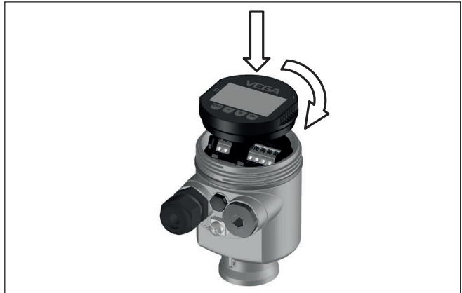
Fig. 5: Installing the display and adjustment module in the electronics compartment of the single chamber housing
