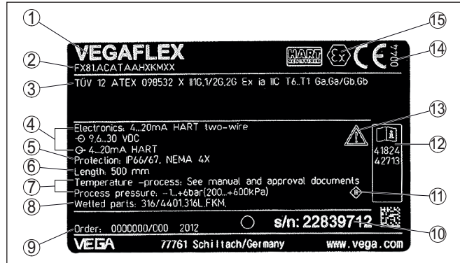
Fig. 1: Layout of the type label (example)
