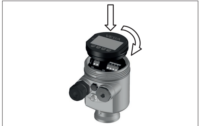
Fig. 10: Installing the display and adjustment module in the electronics compartment of the single chamber housing
