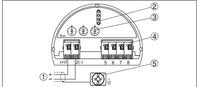
Fig. 3: Electronics and connection compartment - single chamber housing
