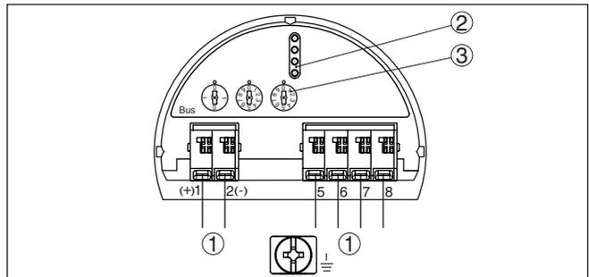
Fig. 4: Electronics compartment - double chamber housing
