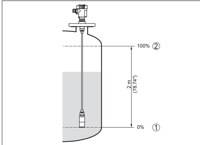
Fig. 8: Parameter adjustment example Min./max. adjustment, level measurement
