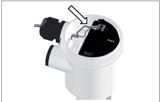
Fig. 2: Connection steps 5 and 6 - Single chamber housing
