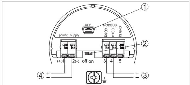
Fig. 14: Compartiment de raccordement
