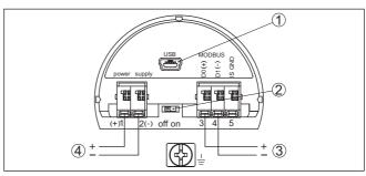
Fig. 11: Connection compartment
