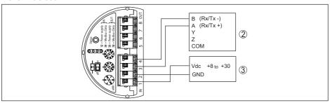
Fig. 27: Connection of VEGABAR 86 to RTU Fisher ROC 809
