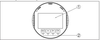
Fig. 16: Display and adjustment elements
