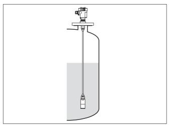
Fig. 2: Level measurement with VEGABAR 86
