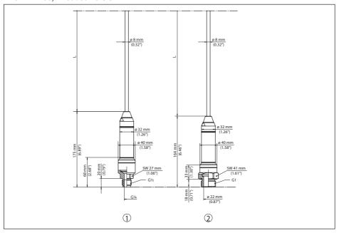
Fig. 36: VEGABAR 86, threaded version
