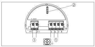
Fig. 10: Electronics compartment - double chamber housing
