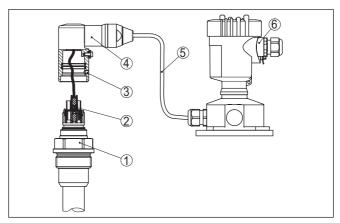
Fig. 24: VEGABAR 86 in IP68 version, 25 bar and lateral cable outlet, external housing
