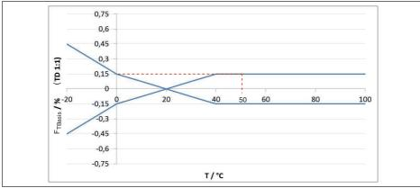
Fig. 28: Determination of the basic temperature error for the above example:  $F_{TRansis} = \frac{0.15 \%}{100}$
