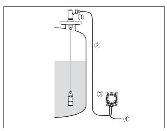
Fig. 7: Arrangement measurement loop, external housing
