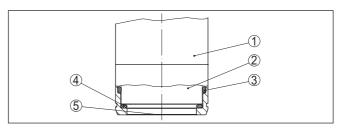
Fig. 3: Front-flush installation of the ceramic measuring cell with double seal
