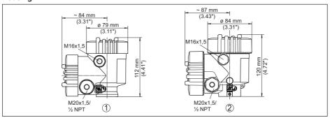
Fig. 29: Dimensions of housing (with integrated display and adjustment module the housing is 9 mm/0.35 inches or 18 mm/0.71 in higher)
