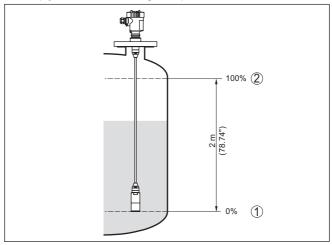
Fig. 18: Parameter adjustment example Min./max. adjustment, level measurement
