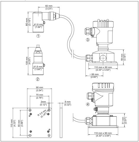
Fig. 30: VEGABAR 86, IP68 version with external housing
