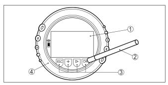
Fig. 17: Display and adjustment elements - with adjustment via magnetic pen
