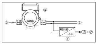
Fig. 21: Connection of the PC via the interface adapter to the RS 485 cable
