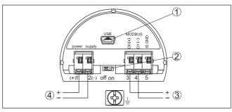
Fig. 14: Connection compartment
