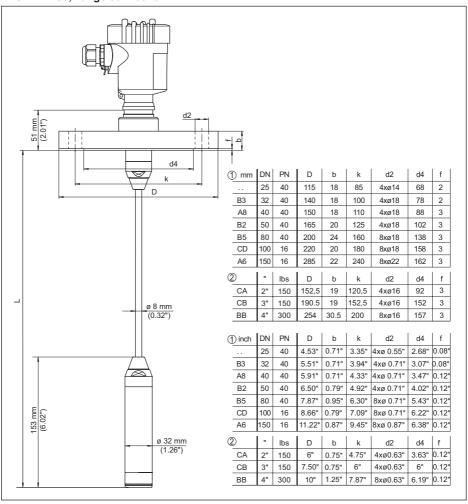
Fig. 34: VEGABAR 86, flange connection
