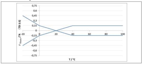
Fig. 26: Basic temperature error F<sub>TBasis</sub> at TD 1:1
