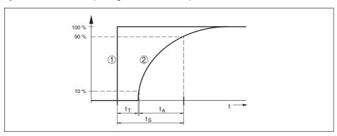
Fig. 25: Behaviour in case of sudden change of the process variable.  $t_{\tau}$  dead time;  $t_{s}$ : rise time;  $t_{s}$ : jump response time
