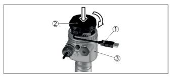
Fig. 19: Connection of the PC directly to the sensor via the interface adapter
