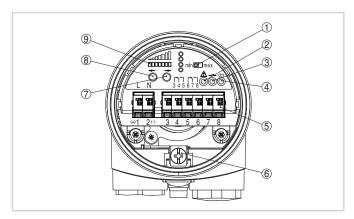
Electronics module receiving unit MP60EE.R - Relay output
