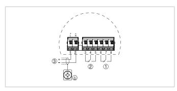
Wiring plan, Receiving unit - VEGAMIP R62 R (receiver)
