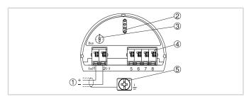
Electronics and connection compartment, single chamber housing
