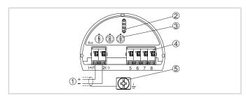
Electronics and connection compartment, single chamber housing
