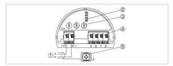
Electronics and terminal compartment, single chamber housing
