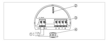
Electronics and terminal compartment, single chamber housing
