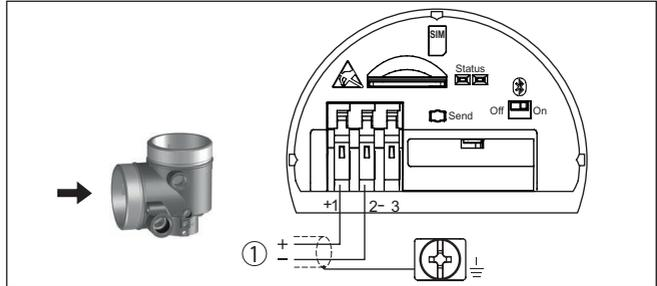
Fig. 16: Compartiment de raccordement - Module radio PLICSMOBILE 81
