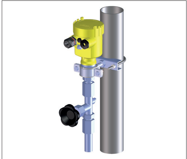
Fig. 15: Mounting example measuring instrument holder
