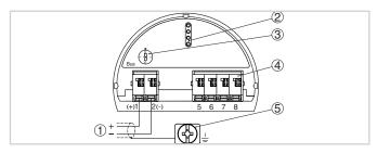
Electronics and terminal compartment, single chamber housing
