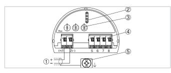
Electronics and terminal compartment, single chamber housing
