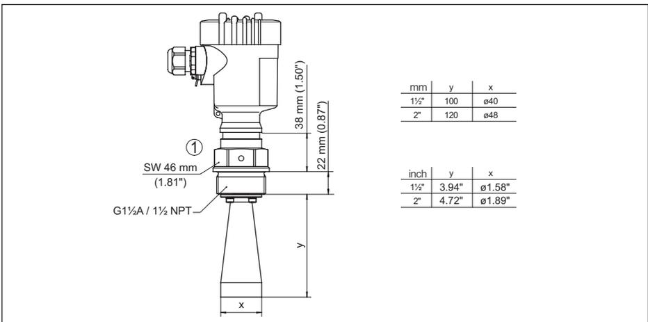
Abb. 38: VEGAMIP 62, Hornantenne (316L)
