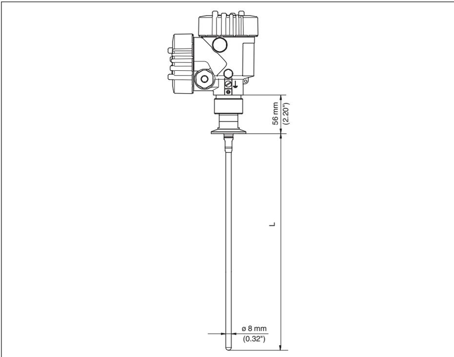
Fig. 36: VEGAFLEX 83, version tige  $\varnothing$  8 mm (0.315 in), polie
