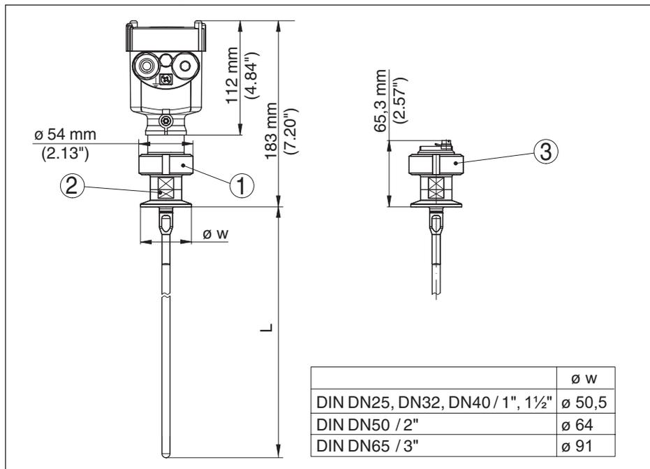
Fig. 37: VEGAFLEX 83, version tige  $\varnothing$  8 mm (0.315 in), polie - Version autoclavée
