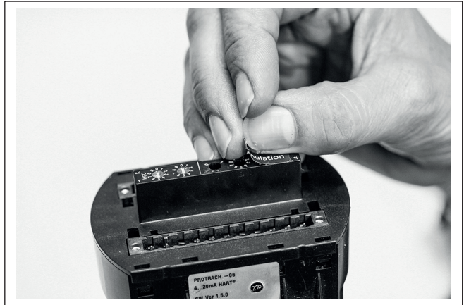
Fig. 2: Profibus PA - Remove the cover foil above the address selection switches
