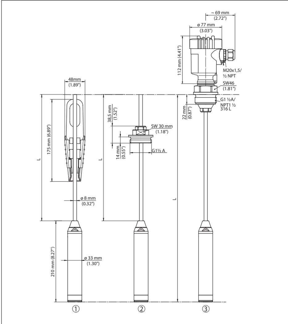
Fig. 17: VEGAWELL 52, with transmitter 316L/Titanium 33 mm
