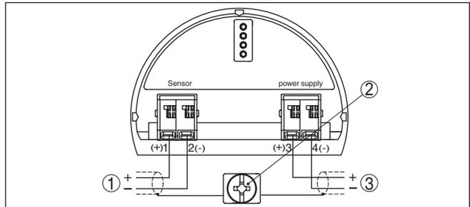
Fig. 13: Wiring plan VEGAWELL 52 for 4 ... 20 mA sensors
