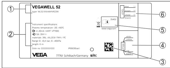
Fig. 2: Layout of the type label (example)
