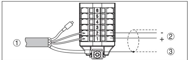
Fig. 11: Wiring plan VEGAWELL 52 4 ... 20 mA, 4 ... 20 mA/HART
