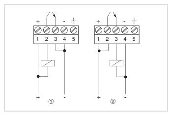
Electronics with transistor output
