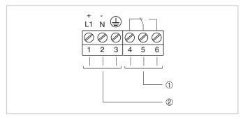
Electronics with relay output
