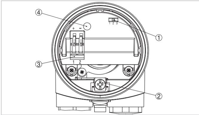
Electronics module - Two-wire output
