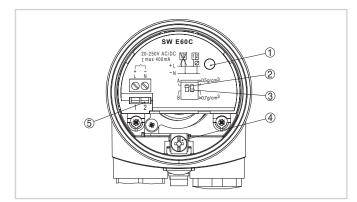
Electronics and connection compartment, single chamber housing
