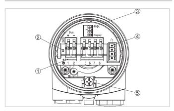
Electronics and terminal compartment, single chamber housing
