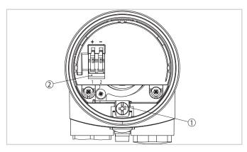
Electronics and terminal compartment, single chamber housing
