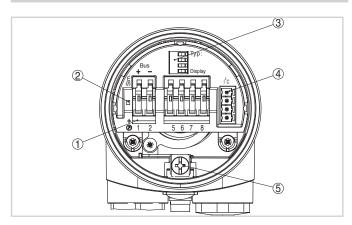
Electronics and terminal compartment, single chamber housing
