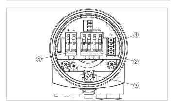
Electronics and terminal compartment, single chamber housing
