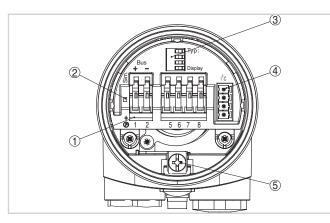
Electronics and terminal compartment, single chamber housing
