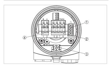
Electronics and terminal compartment, single chamber housing
