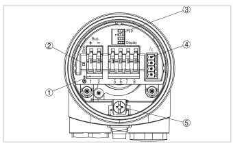
Electronics and terminal compartment, single chamber housing
