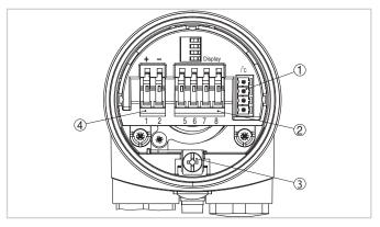
Electronics and terminal compartment, single chamber housing
