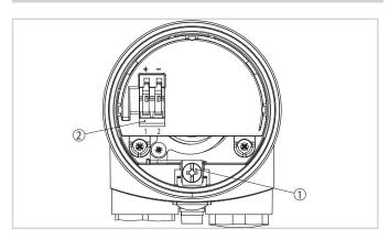
Electronics and terminal compartment, single chamber housing
