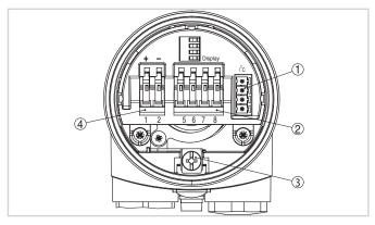
Electronics and terminal compartment, single chamber housing
