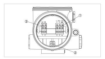
Connection compartment, double chamber housing
