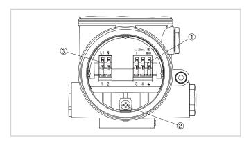
Connection compartment, double chamber housing
