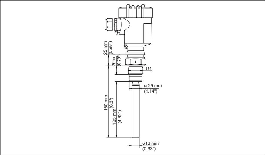
Fig. 20: VEGAVIB 61 - version fileté G1 (DIN ISO 228/1)
