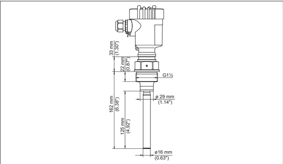
Fig. 21: VEGAVIB 61 - version fileté G1½ (DIN ISO 228/1)
