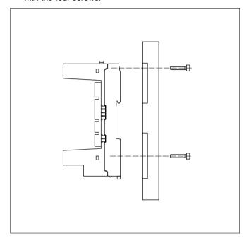
3 Mount the plug-in socket with adapter plate above the four holes to the mounting location
