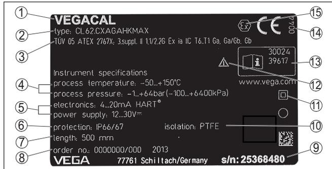
Fig. 2: Layout of the type label (example)
