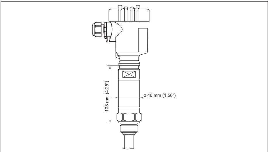
Fig. 35: Temperature adapter
