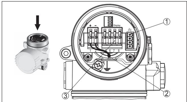
Fig. 17: Electronics compartment - double chamber housing
