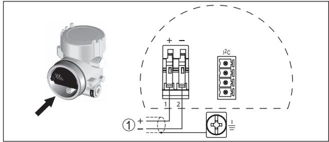
Fig. 15: Wiring plan - double chamber housing
