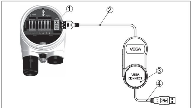
Fig. 24: Connection via interface adapter VEGACONNECT external
