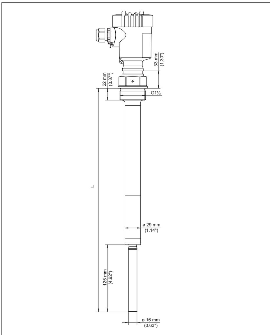
Fig. 19: VEGAVIB 63, Modelo com rosca G1½ (DIN ISO 228/1)
