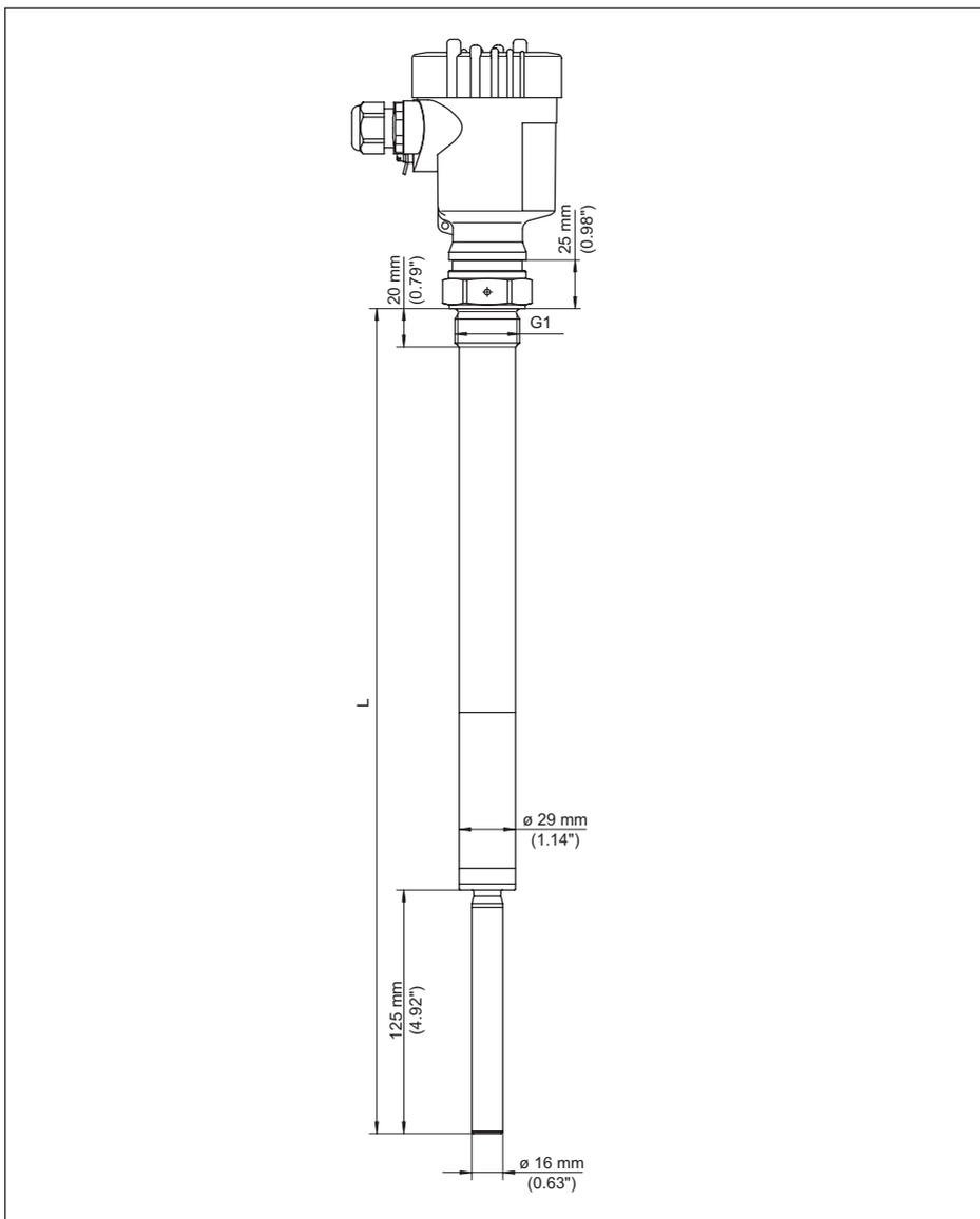
Fig. 18: VEGAVIB 63, Modelo com rosca G1 (DIN ISO 228/1)
