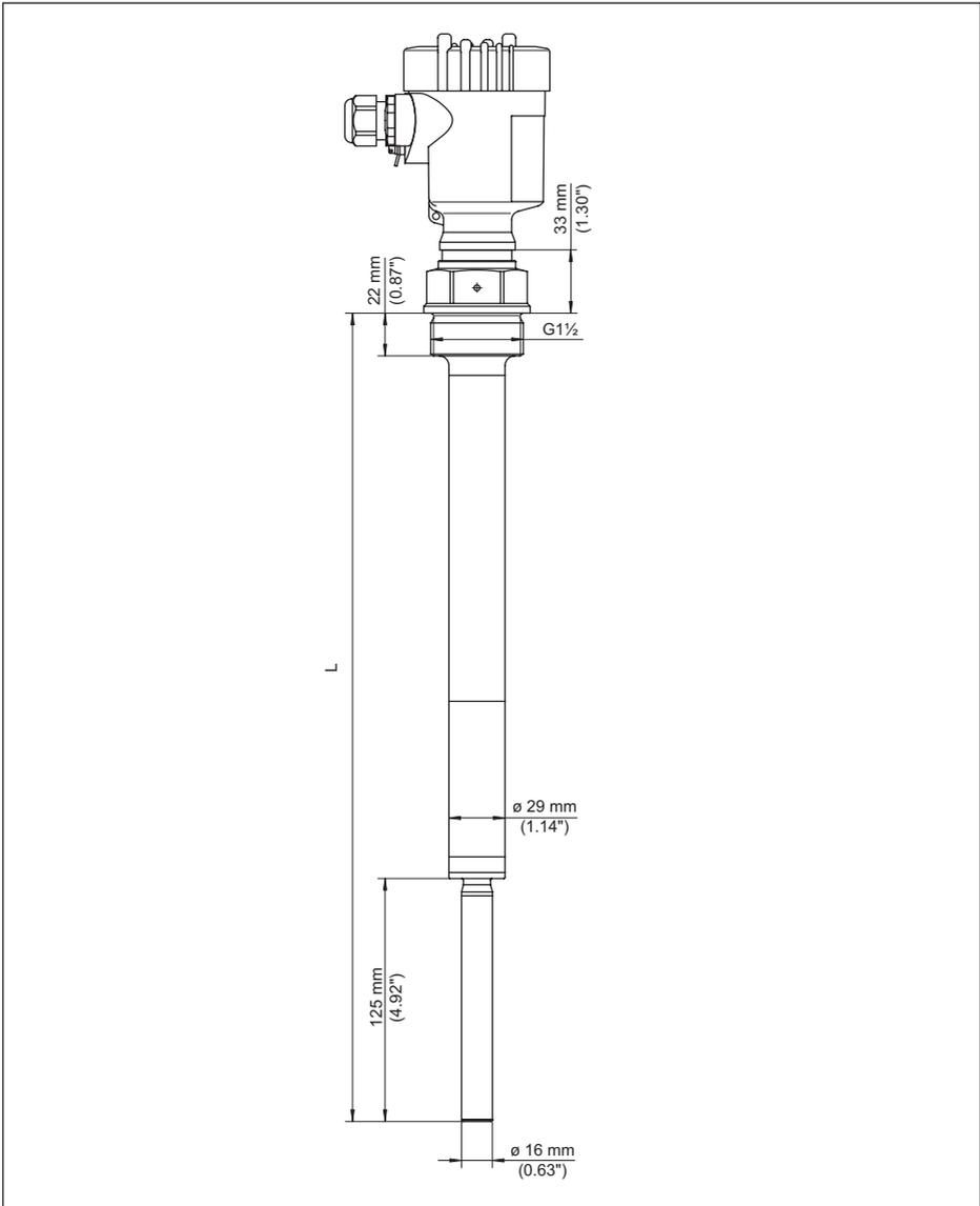
Fig. 20: VEGAVIB 63, Modelo com rosca G1½ (DIN ISO 228/1)
