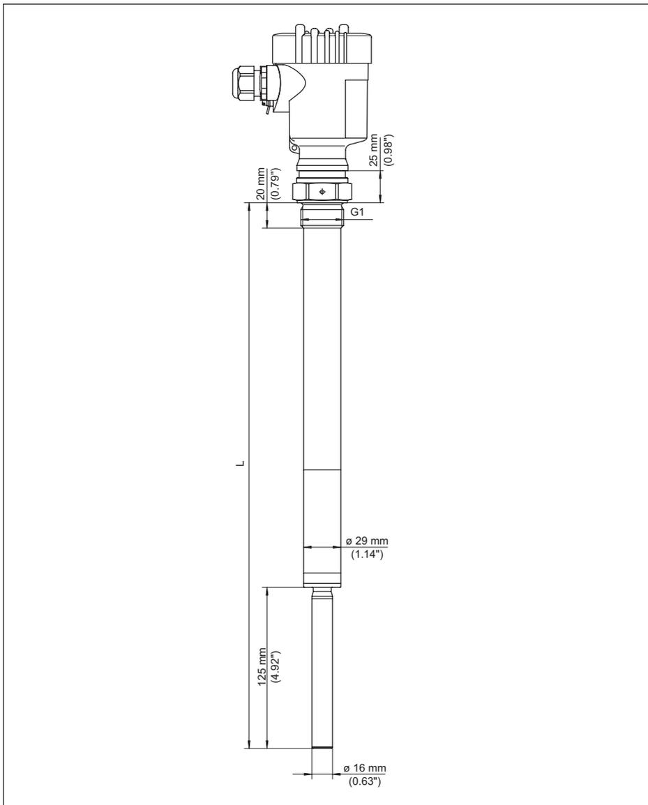
Fig. 19: VEGAVIB 63, Modelo com rosca G1 (DIN ISO 228/1)
