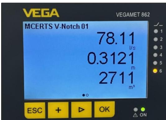
Example of three flow measurement values being displayed on a VEGAMET 86x controller.
