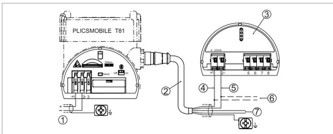
Connection of the voltage supply in the electronics housing
