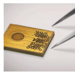
The radar chip inside VEGAPULS 6X combines all our application know-how and the experience gained from 30 years of radar level measurement engineering.
